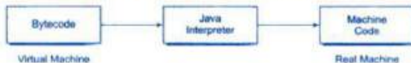
Fig. 3.7 Process of converting bytecode into machine code
